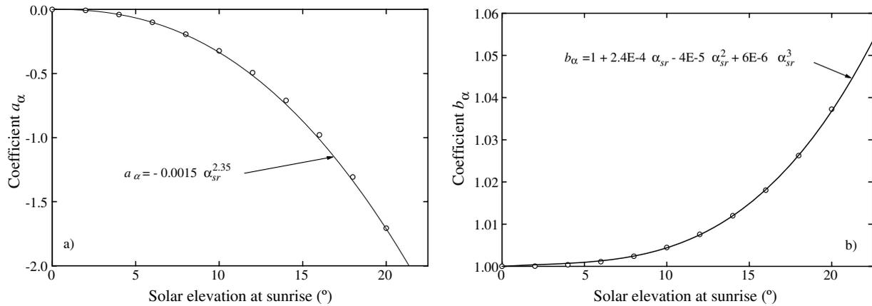
Fig. 3. Dependence of coefficients  $a_\alpha$  and  $b_\alpha$  from Eq. (11) on solar elevation.
