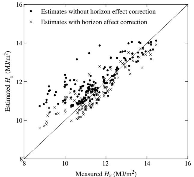
Fig. 6. Estimated without and with the horizon effect term versus measured daily global solar irradiation values for the eleven radiometric stations located in the mountain region of Huéneja (Spain).
