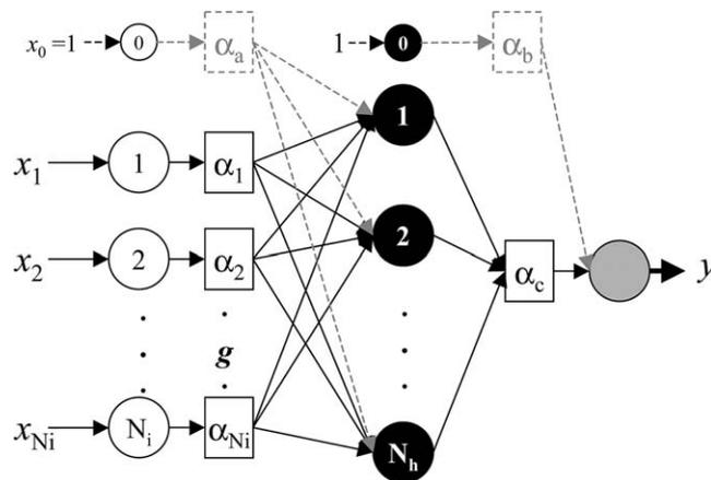
Fig. 2. Graphical representation of the multilayer perceptron with automatic relevance determination. The hyperparameters  $\{\alpha_1, \dots, \alpha_{N_i}\}$  control the weights connecting each input to the hidden layer.
